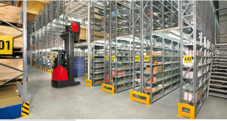
The warehouse has a ground surface area of 900 square metres and is divided up almost quadratically. This manual order picking warehouse has a 3-tier META HIGH-CLIP<sup>®</sup> shelving system.
