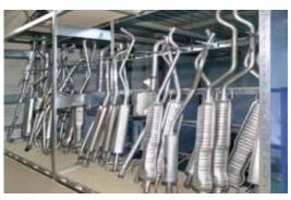
Exhaust pipes tidily arranged and separated by rod dividers
