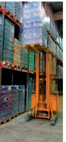
MULTIPAL® bay loads: The frame load data refer to racks with a maximum height of 8 metres (highest beam), up to 12 m on request.
