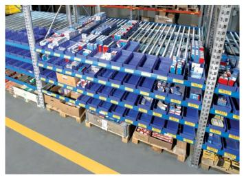
The flow rack levels can be individually adapted to a very wide variety of container sizes
