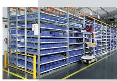
META MULTILINE<sup>®</sup> L order picking flow rack with the FIFOprinciple (First In First Out)
